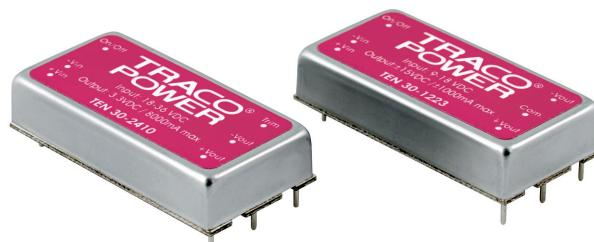
The TEN-30 series is the latest generation of high performance dc-dc converter modules setting a new standard concerning power density. This product with 30W comes in an encapsulated, shielded metal package with a footprint of only 1.0" x 2.0". All models have wide 2:1 input voltage range and precisely regulated, isolated output voltages. Advanced circuit topology provides high efficiency up to 91% which allows an industrial operating temperature range of -40°C to +85°C (with derating).
